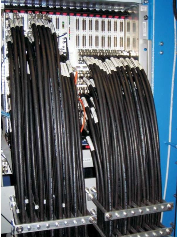
Fig. 8. Photograph of the MUCTPI in the ATLAS underground counting room. Eight MIOCT modules (on the right side) still have to receive their input cables.
