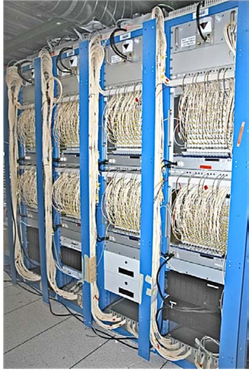
Fig. 11. Liquid argon calorimeter RODs in USA15. 192 RODs housed in 16 VME64 \times 9U crates readout 1524 128-channel front-end boards.
