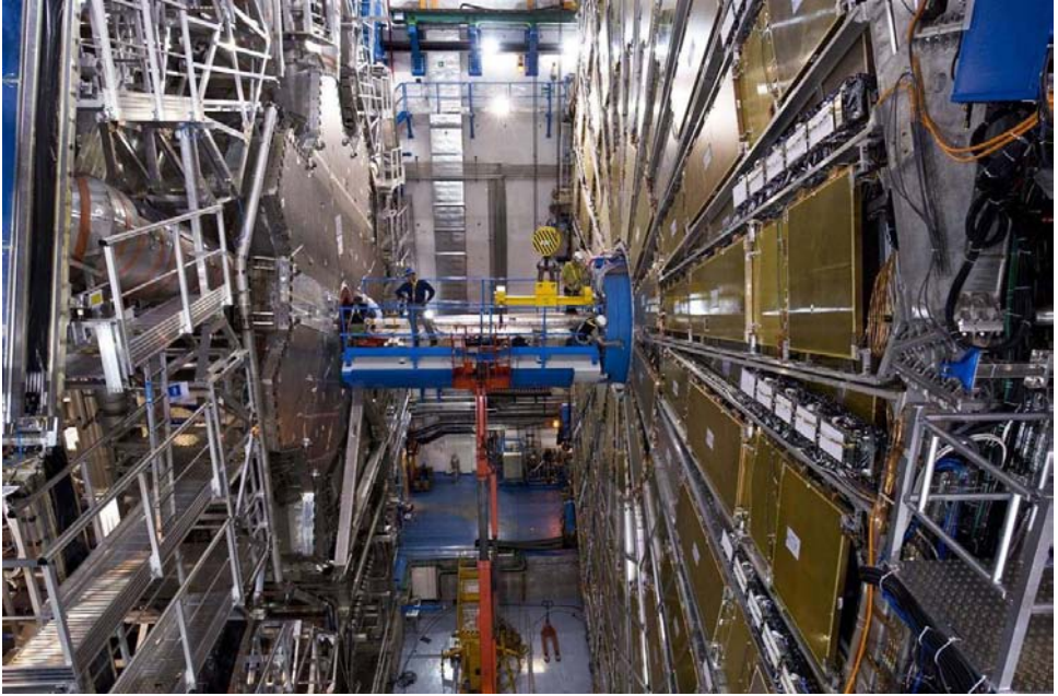
Fig. 22. Closing the beam pipe to prepare for running with the beam. On the left is the front plane of the barrel toroid and end-cap toroid on one side of the experiment, in the center are the beam pipe and radiation shielding segments, and on the right is the first large muon wheel.
