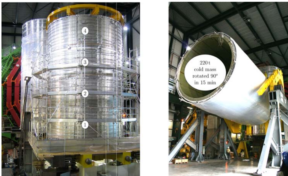
Fig. 8. Left: View of the cold mass with four out of five modules stacked. Right: View of the cold mass with the horizontal axis ready to be inserted in the cryostat.
