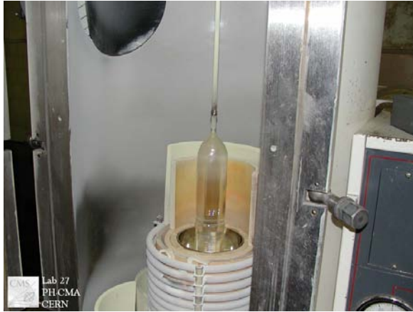
Fig. 3. Picture of a BTCP oven, at the end of a CMS crystal growing cycle ( courtesy of BTCP ).
