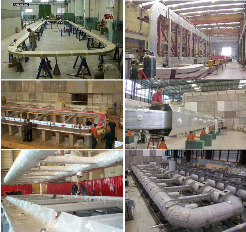
Fig. 10. Production stages of the barrel toroid coils. From top to bottom, left to right: Finishing of a vacuum-impregnated double pancake; assembly by welding of the Al-5083 coil casing; insertion gluing under prestress of the double pancakes in the coil casing; installation of segmented thermal shield panels around cold mass; cold mass insertion in the bottom part of the vacuum vessel; finished coil being prepared for acceptance testing.
