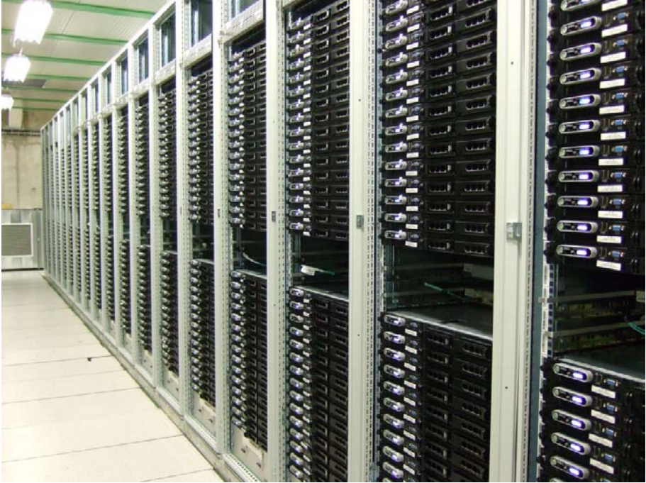
Fig. 7. Part of the ATLAS HLT farm. Each of the one-unit box is a dual-process quad-core computer. There are 31 PCs per rack.
