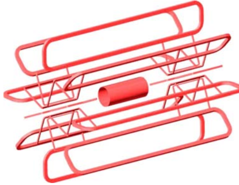
Fig. 4. Layout of the bare windings of the ATLAS magnet system. One can distinguish the solenoid in the center enclosed by the eight barrel toroid coils and the two sets of eight end-cap toroid coils at either end of the solenoid generating bending muon power in low angle forward and backward directions.
